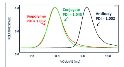
Biopolymer and ABC conjugate are manufactured to high quality with tight molecular weight distribution as shown by PDI
